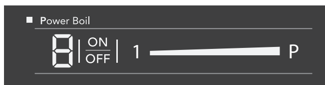
Figure 12: Induction cooking zone control
