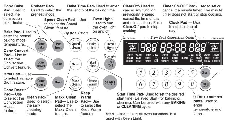
**NOTE**: All instructions are given for the **UPPER oven**. If **LOWER oven** is used the indicator lights will appear in the right portion of the display.
