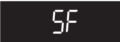
Figure 34: Display showing Sabbath failure
