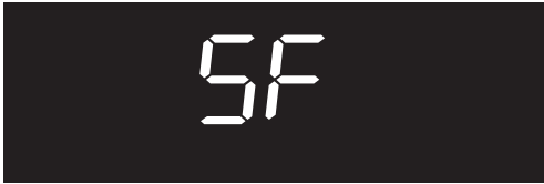
Figure 28: Display showing Sabbath failure
