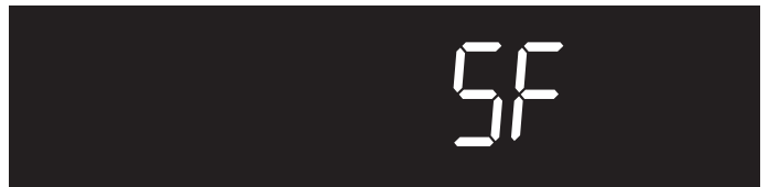
Figure 16: Display showing Sabbath failure
