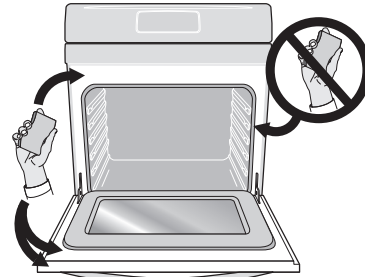
Figure 35: Clean around the oven door gasket
