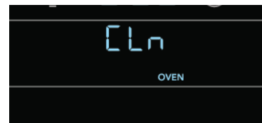
Figure 37: Clean lock icon blinks as door unlocks
