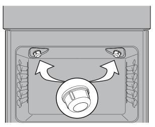
Figure 22: Oven Halogen light
