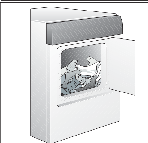
Fill dryer drum 1/3 to 1/2 full.
