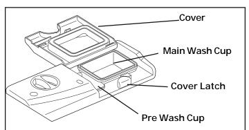
If the cover is closed on the Main Wash Cup, open by pressing the cover latch.
