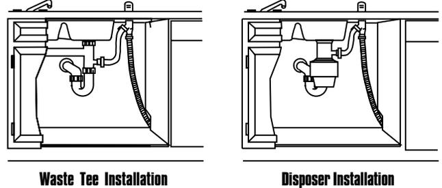
Method 2 - High drain loop with waste tee or disposer
