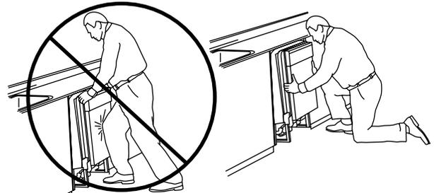
Do Not Push Against Front Door Panel With Knee. Damage to The Door Panel Will Occur.
