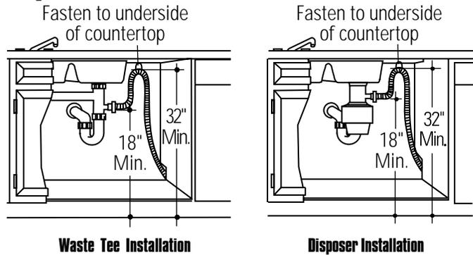
**IMPORTANT** - When connecting drain line to disposer, check to be sure that drain plug has been removed. **DISHWASHER WILL NOT DRAIN IF PLUG IS LEFT IN PLACE.**
