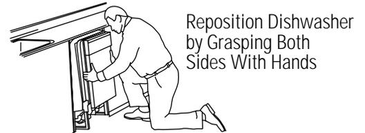
Do Not Push Against Front Door Panel With Knee. Damage to The Door Panel Will Occur.
