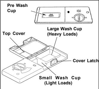
Note: If the cover is closed on the Main Wash Cup, open by pressing the cover latch.
