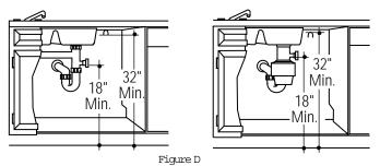
Install waste tee or disposer and air gap according to manufacturer's instructions.
