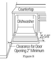
Note: ADA installation. (32-1/2") beneath 34" high counter-tops may be accomplished by adjusting the toekick and leveling legs.
