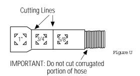
If a longer drain hose is required, add up to 42" of length for a total of 10 ft. to the factory installed hose. Use 5/8" or 7/ 8" inside diameter hose and a coupler to connect the two hose ends. Secure the connection with hose clamps.
