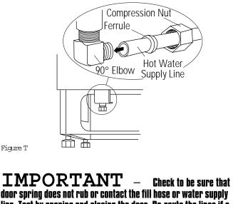
door spring does not rub or contact the fill hose or water supply line. Test by opening and closing the door. Re-route the lines if a rubbing noise or interference occurs.
