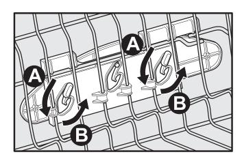
To lower the upper rack, lift the rack straight upward and push rack slightly towards the rear of the dishwasher as it is lowered.
