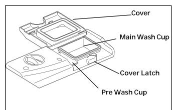
If the cover is closed on the Main Wash Cup, open by pressing the cover latch.
