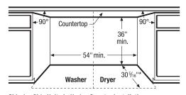
Side-by-Side Units in Under-Counter Installation
