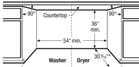
**Side-by-Side Units in Under-Counter Installation**
