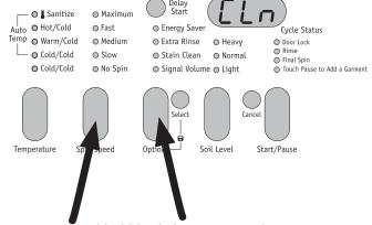
Press and hold both for ten seconds to enter System Clean cycle.
