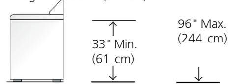
**NOTE:** For installations requiring a longer drain hose, have a qualified technician install a longer drain hose (according to your model number) available from an authorized parts distributor. For drain systems in the floor, install a syphon break kit available from your local hardware store.
