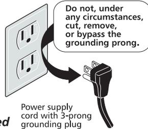
Power supply cord with 3-prong grounding plug
