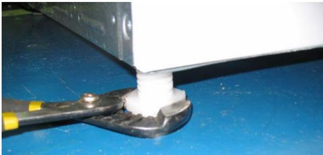
Press down on alternate corners and sides and feel for the slightest movement. Adjust the appropriate leg so the washer is **SOLID** on the floor on **ALL** four legs. Keep the leveling leg extension at a minimum for best performance of the washer.
