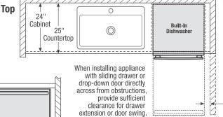
When installing appliance with sliding drawer or drop-down door adjacent to wall, cabinet, or other obstruction that extends beyond front edge of appliance, allow 2" minimum clearance between drawer or door and obstruction.
