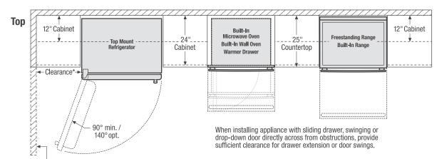
\*When installing top mount refrigerator adjacent to wall, cabinet or other appliance that extends beyond front edge of unit, 20" minimum clearance recommended to allow for optimum 140° door swing, providing complete crisper access and removal. (Absolute 3" minimum clearance will ONLY allow for 90° door swing which will provide limited crisper access with restricted removal.)
