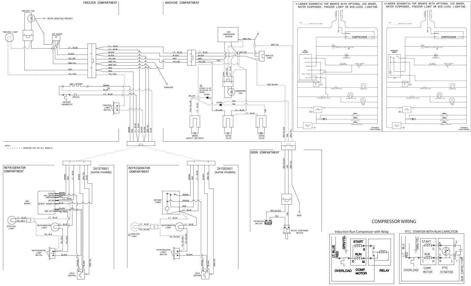
CAPACITOR IS ONLY USED WITH \* SOME P.T.C. MODELS.
