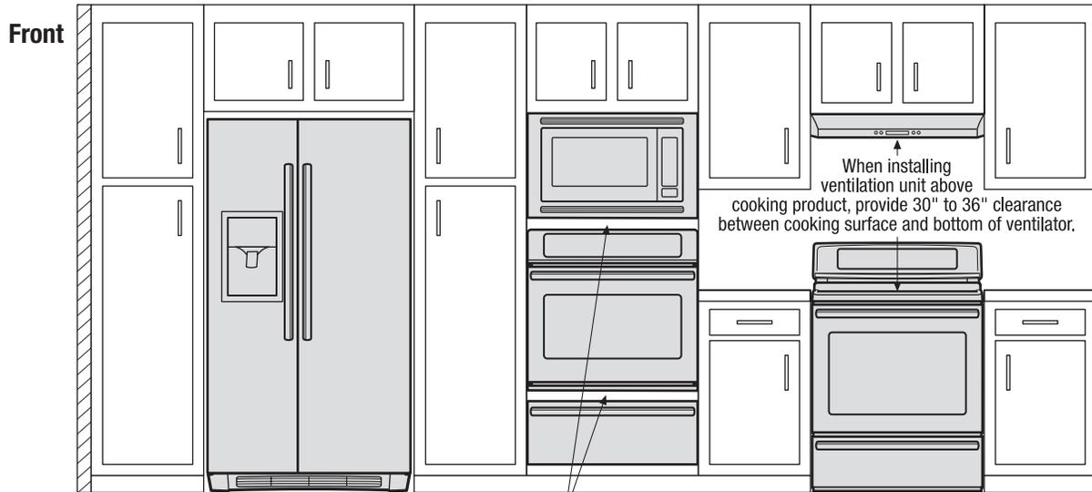
When installing built-in cooking appliances in combination, 2"-high minimum visible gap between appliance faceplates required.
