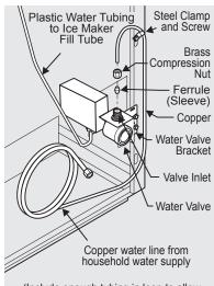
(Include enough tubing in loop to allow moving refrigerator out for cleaning.)
