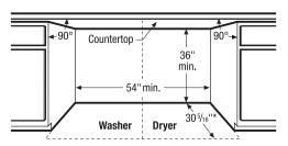
Side-by-Side Units in Under-Counter Installation
