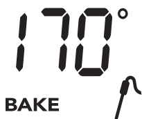
Figure 18: Probe set showing probe temperature
