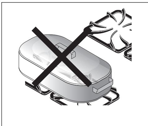
**Wire trivets:** Do not use wire trivets. Cookware bottoms must be in direct contact with the grates.
