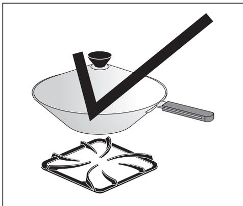
**Woks** with flat bottoms suitable for use on your cooktop are available in most cookshop or hardware stores. Round-bottomed woks (with a support ring that does not extend beyond the burner unit) may also be used. The metal ring was designed to support the wok safely when it is filled with large amounts of liquids (soup making) or fat (frying).
