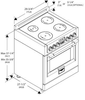
• Within 3" (7.6 cm) side clearance, wall cabinets no deeper than 13" (33.0 cm) must be minimum
