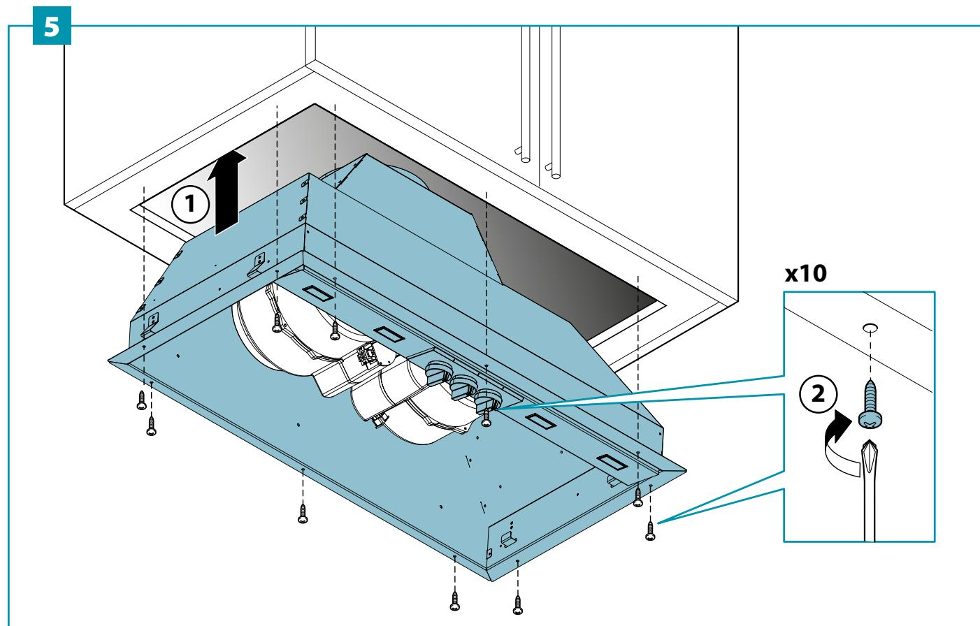
**EN** - Secure frame to hood body (6), insert filters (7).
