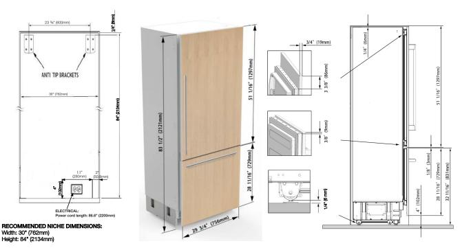
Depth: 25 1/2" (24 3/4" (629mm) + 3/4" panel thickness for flush to gable finish). Alternatively, 25" (when using a recessed receptacle or if receptacle is in an adjacent cabinet kick space).
