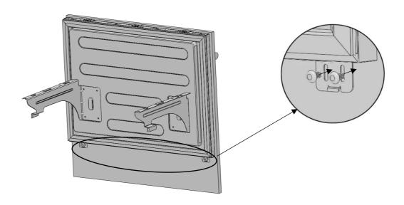
• Clip the door overlay panel bracket cover onto the brackets (Item No14).
