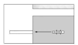
• Fit the anti-tip brackets (item No.2) into their places, using 4 screws (item No.4) for each. You must use both the (2) brackets to ensure the safety of the product.
