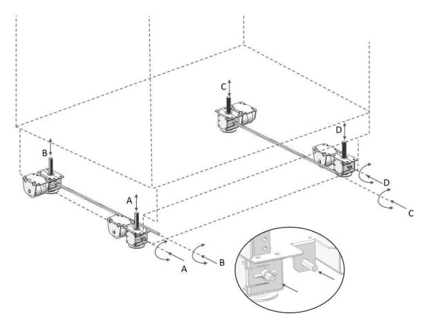
Fist start with raising the front feet (before the back feet) to reduce the risk of the appliance falling frontward.
