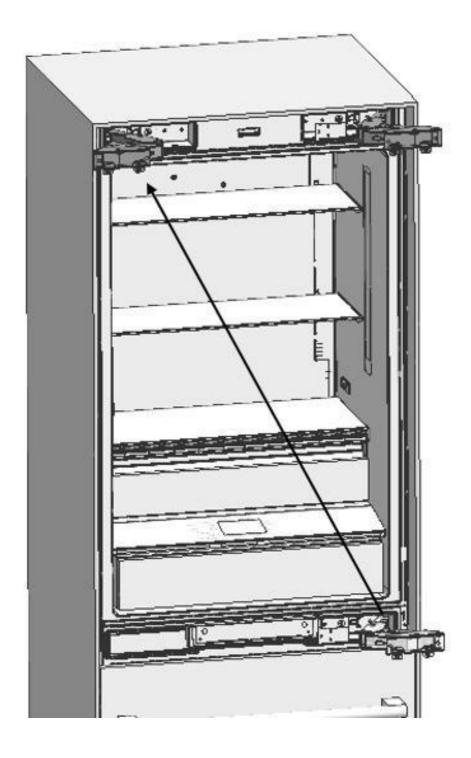
• Remove the upper right hinge by loosening its 2 screws and fix it to its slot at the lower left side.
