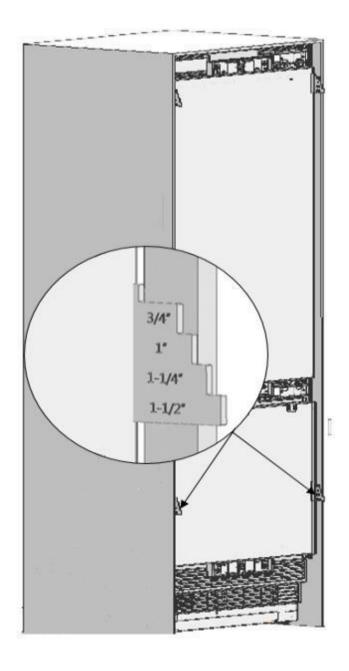
• The position adjustment jig (Item No5) must be adjusted according to the thickness of the door. It can adjust the level for 4 different door thickness levels.
