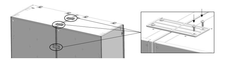
After making sure that they are in alignment screw the lower brackets to the other refrigerator.
