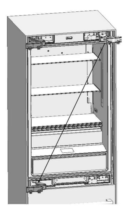
Attach the hinge slot caps removed from the left side to the hinge caps at the right side.
