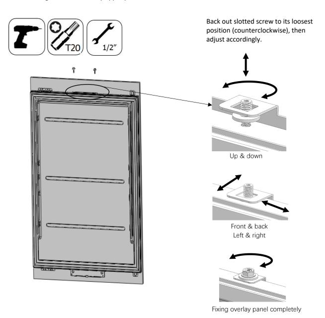
• How to align the door overlay panel lower section with bolts.
