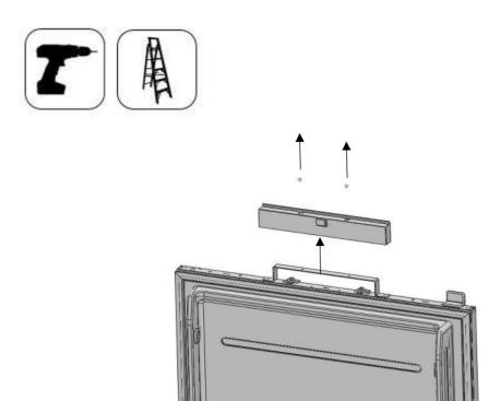
• Loosen 2 screws of the lower cover of the fridge door and remove it.
