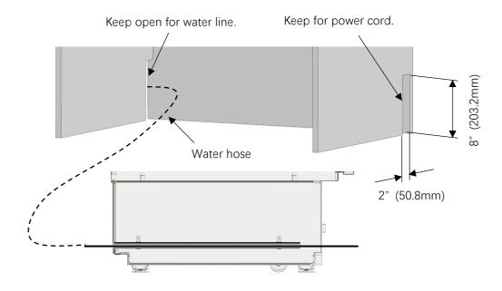
Utilize the factory installed pass-through tube to feed the waterline through to the front where the connection to the valves will be made.
