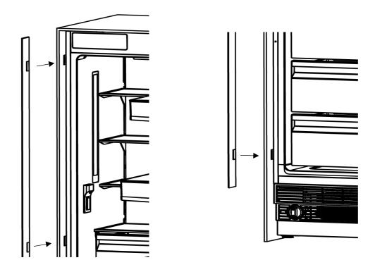
Attach the top trim onto the cabinet-appliance connecting brackets.
