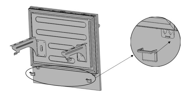
• Install the complete freezer door assembly onto the rails.
