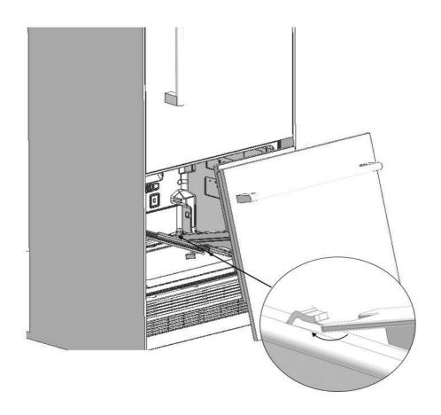
• Once the freezer door assembly is in place, secure to the drawer rails with 2 screws.
