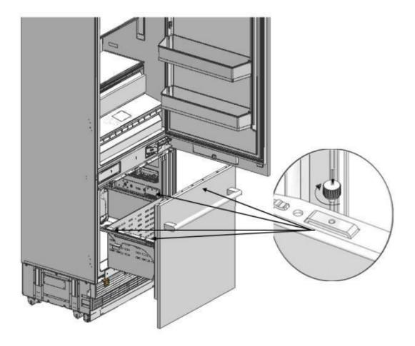
• Snap the freezer drawer cover strip (Item No5) onto the buttons on top of the freezer drawer. It should fit tightly against the overlay panel.
