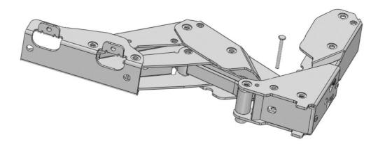
90° limit pin should be inserted to upper hinge and lower hinge
