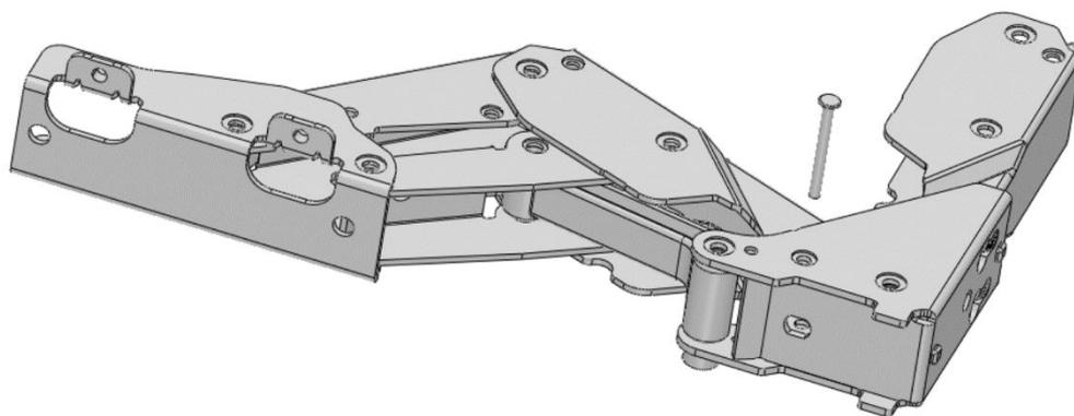
90° limit pin should be inserted to upper hinge and lower hinge
