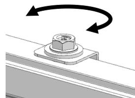
Fixing overlay panel completely
