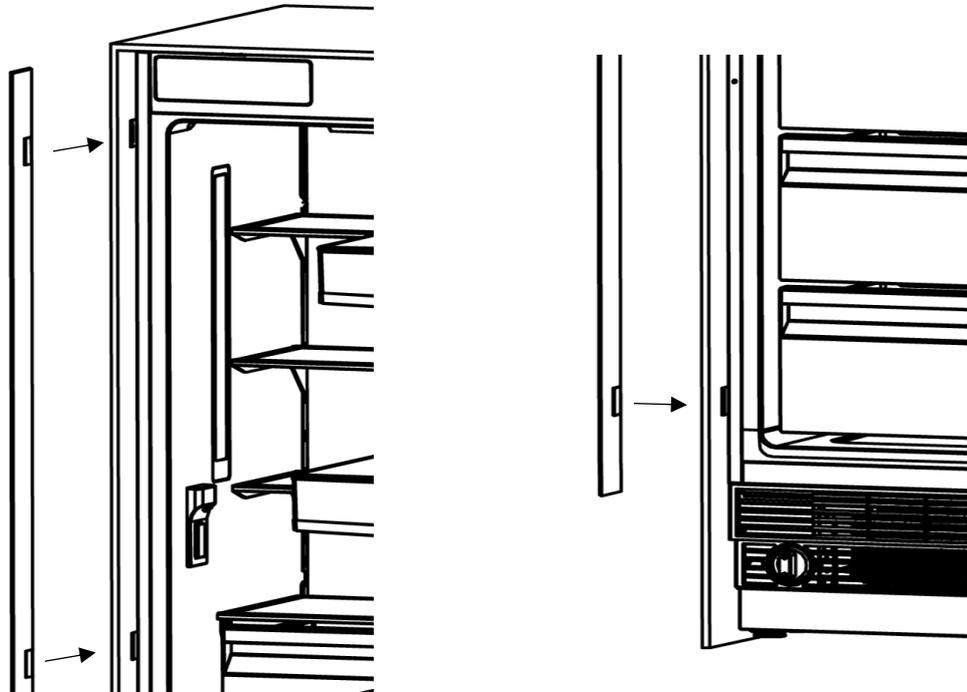
Attach the top trim onto the cabinet-appliance connecting brackets.
