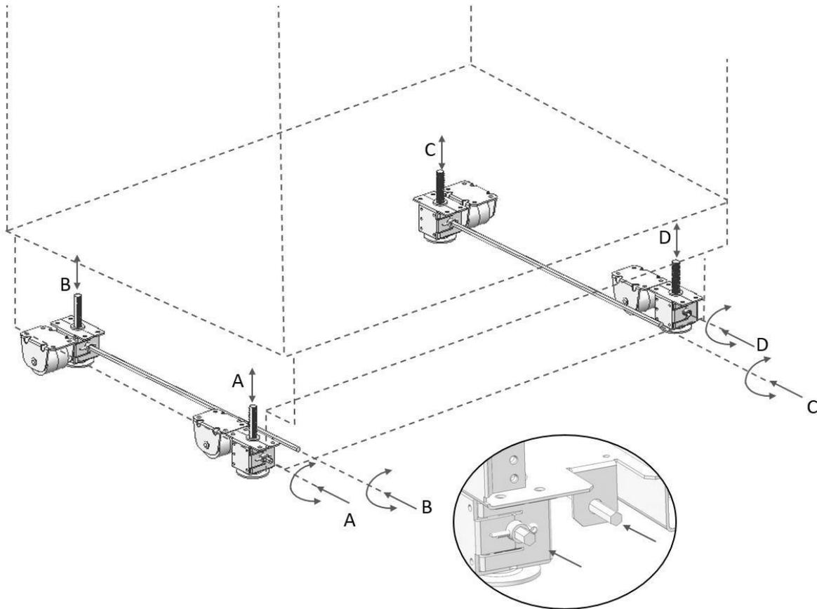
First start with raising the front feet (before the back feet) to reduce the risk of the appliance falling forward.
