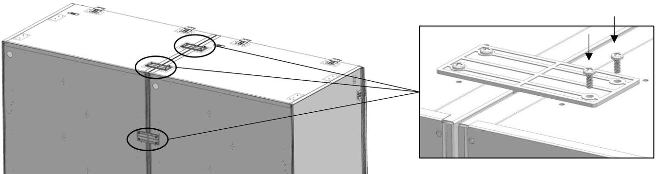
After making sure that they are in alignment screw the lower brackets to the other refrigerator.
