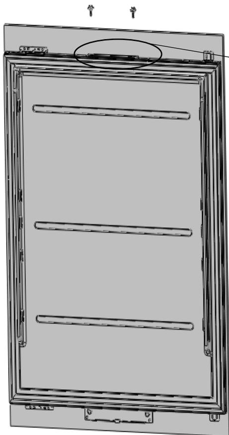
Back out slotted screw to its loosest position (counterclockwise), then adjust accordingly.
