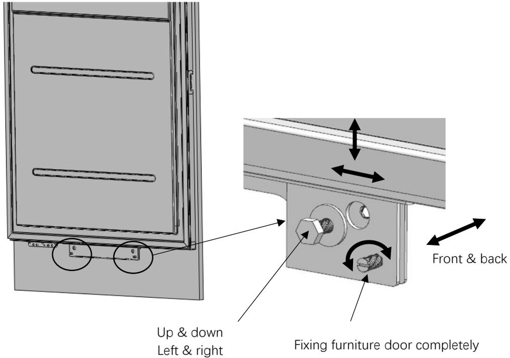
Use the set screws to position the panel in the Z (depth) direction then fix in place firmly with the washers and bolts removed in the earlier steps. Do not over-tighten as it will bend the brackets.
