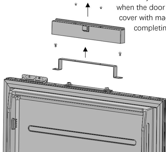
**IMPORTANT:** There is a magnet inserted into this cover that is necessary for the appliance to detect when the door is closed. Ensure this cover with magnet is replaced when completing the installation.
