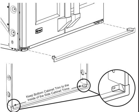
Exercise caution while sliding the unit back in after bottom trim installation. Installer needs to ensure that the trim does not catch the edge of the cabinet and bend. Furthermore, the installer needs to ensure that the cabinet itself is not damaged while the unit is slid back into position.
