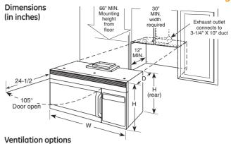
The Spacemaker convection/microwave and Spacemaker microwave ovens are designed for adaptation to the following three types of ventilation:
