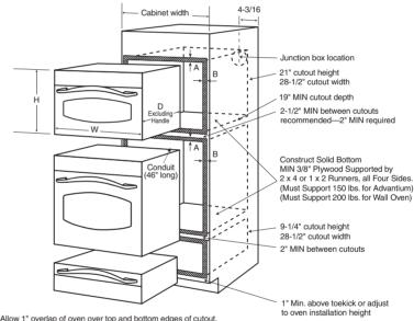
A=Allow 1" overlap of oven over top and bottom edges of cutout. B=Allow 11/16"-3/4" for overlap of oven over side edges of cutout.
