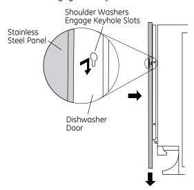
5 Press the panel against the door and push downward until the washers are fully engaged into the keyhole slots. The panel should align evenly with the top and sides.
