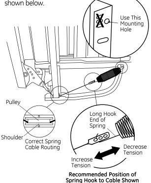
**TIP:** If the door does not open easily or falls too quickly. check spring cable routing. The cable is held in place by "shoulders" on the pulley. Check to be sure the cable has not slipped over the pulley shoulders.
