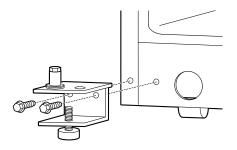
F Remove the insert at the top left side of the base grille and install it on the right side.
