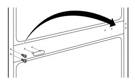
**B** Install the center hinge on the left side.
