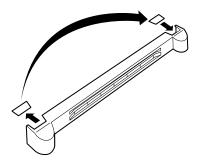
Replace the base grille by aligning the prongs on the back of the grille with the holes in the cabinet. Push forward until the grille snaps into place.
