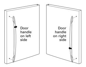
Align keyhole slots on the top and bottom of the back of the handle with the screws mounted on the front of the door. Press the handle against the door front, making sure that the screws go into the keyhole slots.
