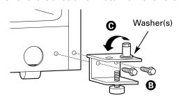
D Using a 3/8" socket driver, remove the leveling leg bracket from the bottom left side of the cabinet and install it on the right side.
