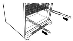
B Locate the slots on the inside of the rail assemblies near the back.
