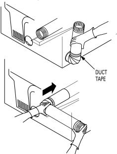
• Apply duct tape as shown on the joint between the dryer internal duct and the elbow.
