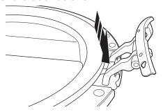
Push the hinge assembly into place until the hinge holes align with the door holes.
