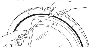
Insert the hinge cover. Align the hinge cover holes with the holes in the door.
