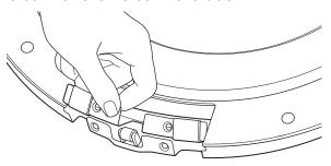
Secure the hinge cover with the 2 tapping screws (#8).
