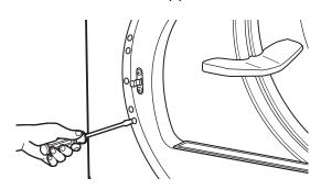
Switch the strike bracket and its cover on the opposite side by removing the screws. Reinstall both on the opposite side.
