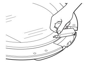
Remove the hinge assembly by removing the 2 machine screws (#8) that fasten it to the frame. Pull the hinge assembly out of its cavity and set it aside.
