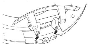
Fasten the hinge assembly to the edge using 2 machine screws (#8).
