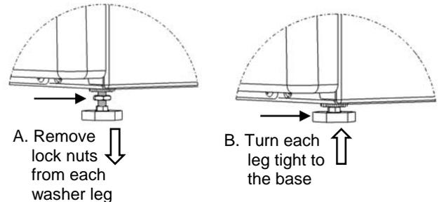
**3** On washer or dryer models with **PLASTIC LEVELING LEGS**, make sure the leveling legs are threaded fully into the base.
