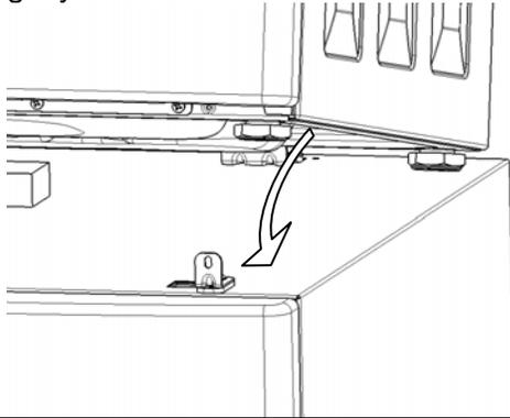
**6** Set the unit down onto the pedestal making sure the base of the unit is behind the front brackets of the pedestal and align bracket hole with base mounting hole.
