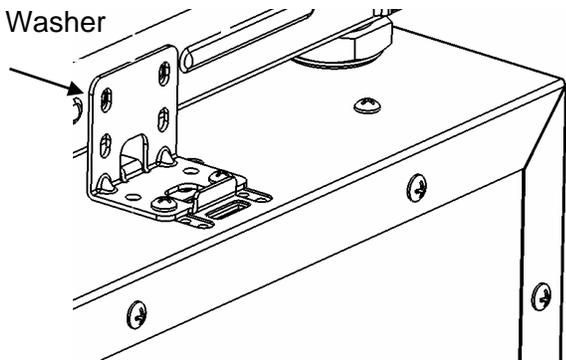
**NOTE:** If slots or mounting holes do not align, make sure the washer or dryer leveling legs are adjusted fully into the unit. Turn each leg tight to the base.
