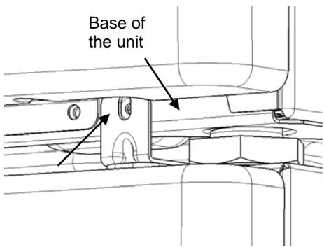
**7.a** For the washer, align the holes in the rear of the washer with the slots of the rear brackets on the pedestal.
