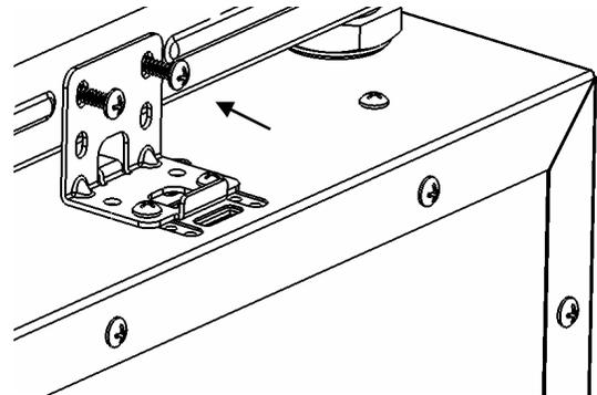
**9** With the pedestal drawer open for better access, install a #10 screw through each front bracket on the pedestal into the base of the washer or dryer.
