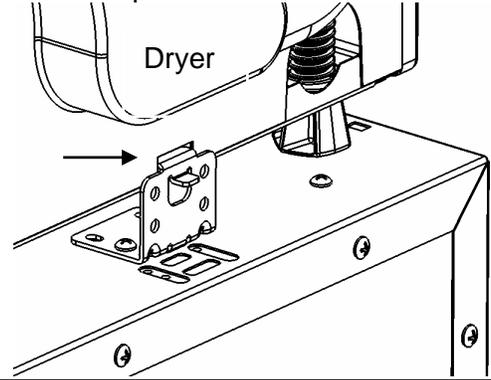
**8** Align the sides of the washer with the sides of the pedestal and secure the washer to the rear brackets using four #10 screws (2 per bracket).
