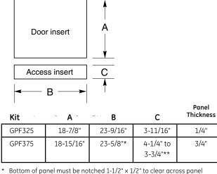
\*\* Adjustment required to match adjacent cabinet fronts due to leveling leg adjustment, 4" nominal
