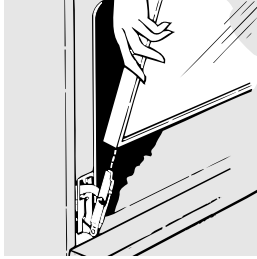
Lift the door straight up and off the hinges.
