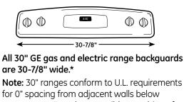
Note: 30" ranges conform to U.L. requirements for 0" spacing from adjacent walls below countertops. To reduce possible scorching of walls, engineering recommends a minimum of 1-1/2" spacing to allow for possible extended, high heat, no-load heating element operation.
