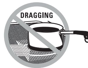
Do not slide cookware across the cooktop because it can scratch the glass—the glass is scratch-resistant, not scratch proof.
