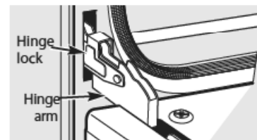
Push hinge locks up to lock.
