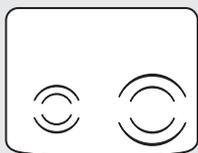
To use the small surface unit, turn the control knob **counterclockwise** to the **SMALL BURNER** settings.
