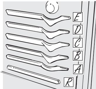
The oven has a special lower rack (R) position just above the oven bottom. Use it when extra cooking space is needed, for example, when cooking a large turkey. The rack is not designed to slide out at this position.
