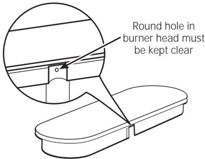
For proper ignition, make sure the small hole in the notch that fits over the electrode is kept open. A sewing needle or wire twist-tie works well to unclog it.
