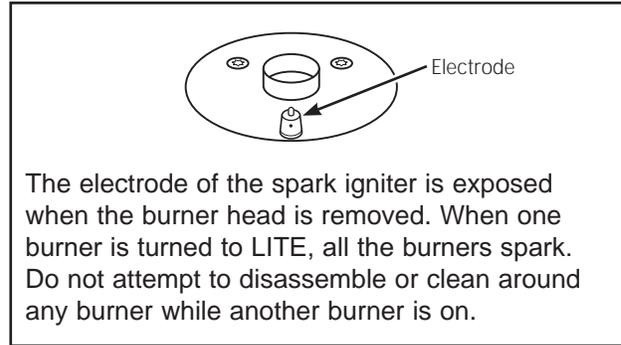
The electrode of the spark igniter is exposed when the burner head is removed. When one burner is turned to LITE, all the burners spark. Do not attempt to disassemble or clean around any burner while another burner is on.
