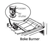
A. If the flames are yellow, open shutter more than the original setting. B. If the flames lift off the burner, close the air
