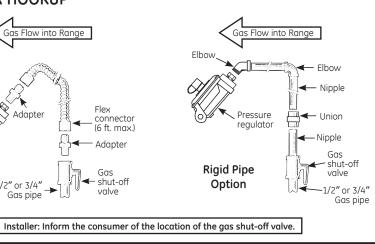
To prevent gas leaks, put pipe joint compound on or wrap pipe thread tape with Teflon\* around, all male (external) pipe threads.
