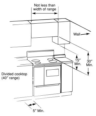
**NOTE:** There is a minimum 5" clearance required from the left side of the range to a wall. This clearance is needed to open the left side oven door or to remove the left oven shelf.
