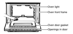
**3.** Clean spatters or soil on the oven front frame and the oven door outside the gasket with a dampened cloth. The oven front frame and the oven door outside the gasket do not get cleaned by the self-clean cycle.
