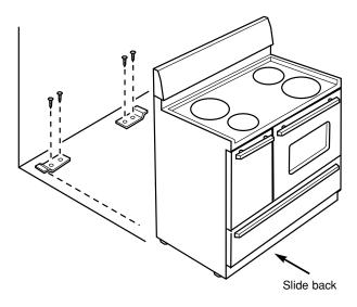
**5.** Slide the range into place making sure the rear legs are trapped by the ends of the brackets. The range may need to be shifted slightly to one side as it is being pushed back to allow the rear legs to align with the brackets. Remove the storage drawer to inspect brackets or grasp the top rear edge of the range and carefully attempt to tilt it forward to make sure the range is properly anchored.
