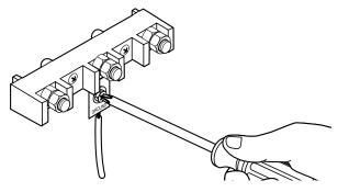
**E.** Remove the three outer terminal nuts from the terminal block.
