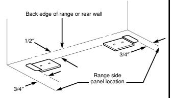
Brackets attach to the floor at the back of the range to hold both rear leg levelers. When fastening to the floor, be sure that screws do not penetrate electrical wiring or plumbing. The screws provided will work in either wood or concrete. **1.** Unfold the paper template and place it flat on the floor with the back and side edges positioned exactly where the back and sides of the range will be located when installed. (Use the diagram to locate the brackets if the template is not available.)
