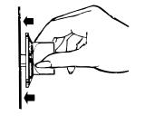
The control must be pushed in to set only from the OFF position. When the control is in any position other than OFF, it may be turned without pushing it in.
