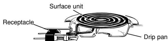
Lift the surface unit about 1 inch above the drip pan and pull it out.
