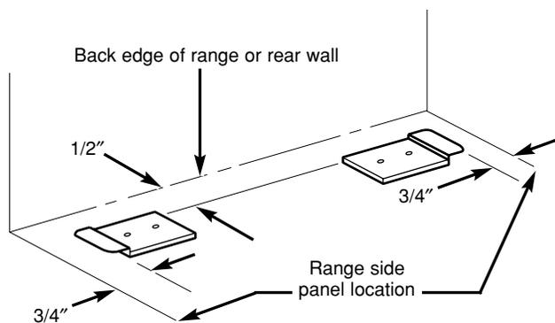
Brackets attach to the floor at the back of the range to hold both rear leg levelers. When fastening to the floor, be sure that screws do not penetrate electrical wiring or plumbing. The screws provided will work in either wood or concrete.
