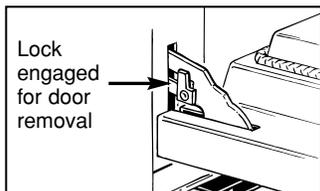
Keep pulling the bottom of the door toward you while pushing the top of the door toward the range. Pull the door free of the hinges.
