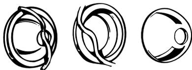
The oven light has a glass lens held in place with a spring wire to protect the oven bulb from the heat of the oven.
