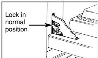
3. Hold the door by the sides. Pull the bottom of the door up and toward you to release it from the hinges.
