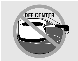
Always place the pan in the center of the surface unit you are cooking on.
