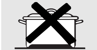
Pans with rounded, curved, ridged or warped bottoms are not recommended.
